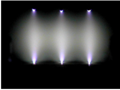
Fig. 40. Parallel operation of MHCS discharges in atmospheric pressure air stabilized by ballast resistors. The electrode gap is 8 mm [116].
