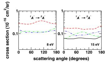
Fig. 17. Differential cross sections for the  $^1A' \rightarrow ^3A'$  electronic excitation of phenol (C<sub>6</sub>H<sub>5</sub>OH) by electron impact at the energies of 8 eV (left panel) and 15 eV (right panel). Dashed (red) line, dash-dotted (green) line, dash-dot-dotted (blue) line and solid (black) line, theoretical results from reference [137] obtained at the 3ch-sep, 8ch-sep, 13ch-sep and 23ch-sep levels of approximation, respectively. Adapted from reference [137].
