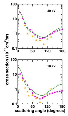
Fig. 4. Differential cross sections for electron scattering by  $CF_3I$  at 30 and 50 eV. Solid line, theoretical results in the static-exchange approximation; diamonds, experimental data from reference [65]; triangles, experimental data from reference [66].
