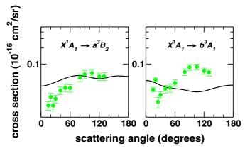
Fig. 15. Differential cross sections for the  $X^1A_1 \rightarrow \tilde{a}^3B_2$  (left panel) and  $X^1A_1 \rightarrow \tilde{b}^3A_1$  (right panel) electronic excitation of furan (C<sub>4</sub>H<sub>4</sub>O) by electron impact at 7.5 eV. Solid line, theoretical results from reference [133] obtained up to the 9ch-sep level of approximation; circles, experimental data from reference [133]. Adapted from reference [133].
