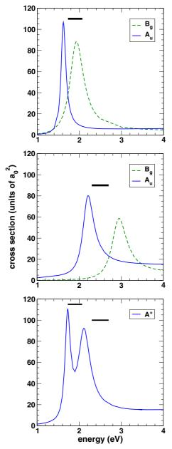
Fig. 7. Integral cross sections for the resonant symmetries of FAD, FD and FAFC. The bars indicate the resonances of HCOOH and of HCONH<sub>2</sub> in the gas phase, which are centered at 1.9 eV and 2.5 eV respectively. The bars width represents the width of the resonances estimated from the calculations.
