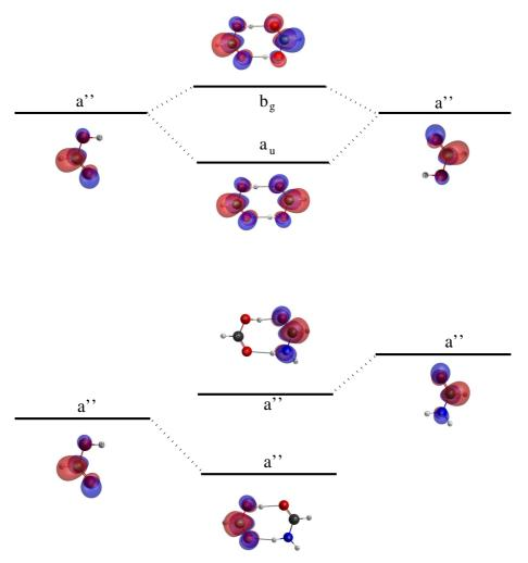
Fig. 8. Model based on the molecular orbital theory showing a pictorial view of the formation of the shape resonances in the FAD, FD and FAFC from the units formic acid and formamide.
