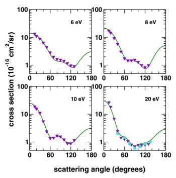
Fig. 1. Differential cross sections for electron scattering by CF<sub>3</sub>Br at 6, 8, 10 and 20 eV. Solid line, theoretical results from reference [61] obtained in the static-exchange approximation; triangles, experimental data from reference [62]; squares, experimental data from reference [63]. Adapted from reference [61].
