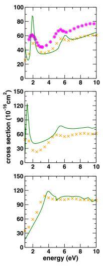
**Fig. 5.** Integral cross sections for electron collisions with SiCl<sub>4</sub> (top), SiBr<sub>4</sub> (middle) and SiI<sub>4</sub> (bottom). We also present the measured total cross sections from reference [68] (crosses) and from reference [69] (stars). Adapted from reference [67].
