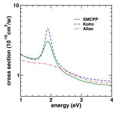
Fig. 6. Differential cross section for electron collisions with formic acid at a scattered angle of 135° as a function of the energy. Solid line, present results; dashed line, results of the complex-Kohn method [90]; dot-dashed line, experimental data of Allan [91].
